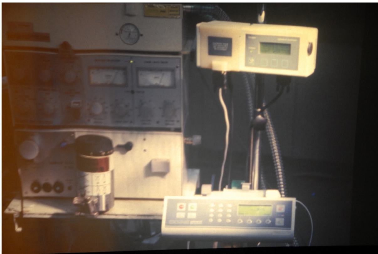
Fig. 1 — Prototype of the Diprifusor® allowing the delivery of propofol TCI using the Marsh pharmacokinetic set.
