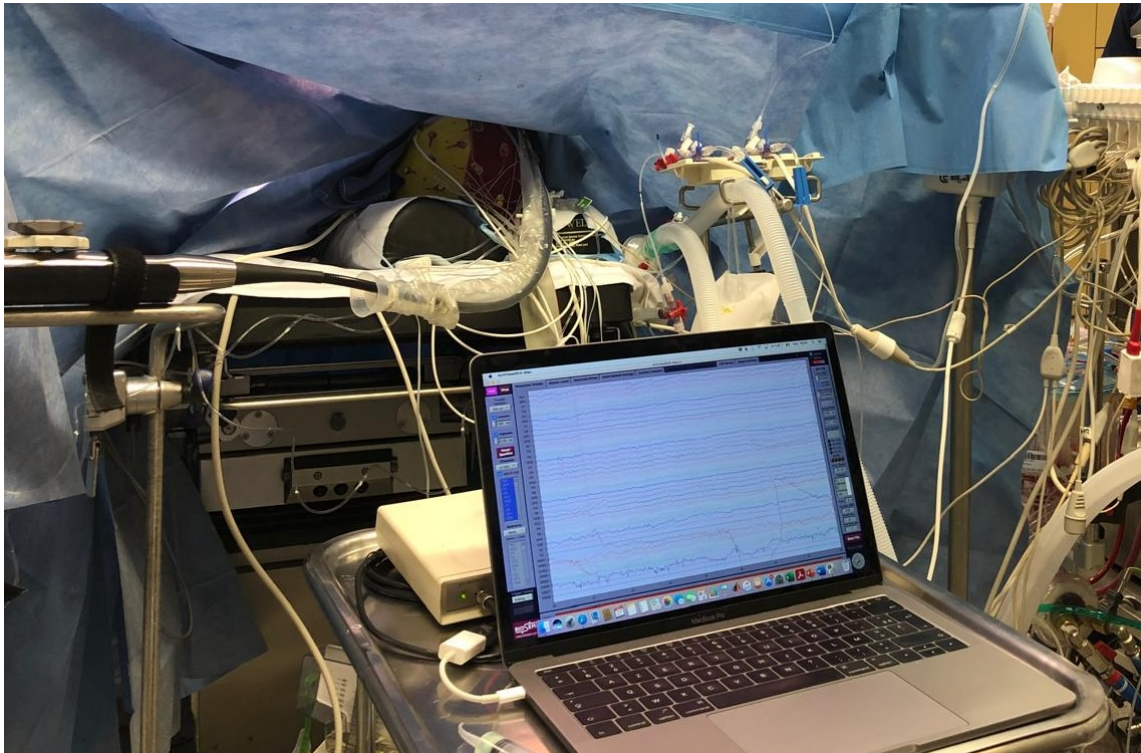
Fig. 2 — Intraoperative setup of the 32-channel BioSemi ActiveTwo electroencephalogram recording system.
